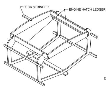
3. Glue Engine Hatch Ledger in position shown 2-Places.
