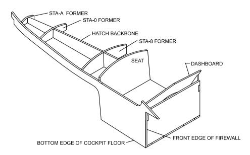
8. - Attach 1/16" plywood side piece lining up to bottom and front of Firewall.
