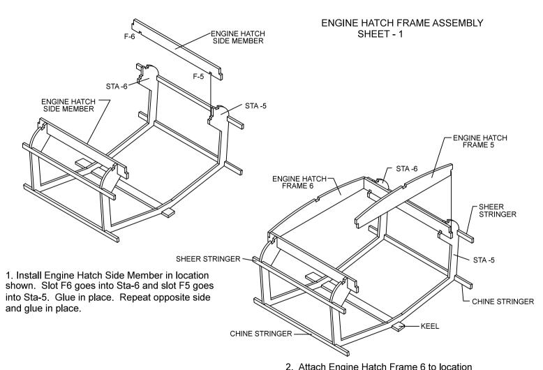
2. Attach Engine Hatch Frame 6 to location shown and glue in place. Repeat with Engine Hatch Frame 5 and glue in place.
